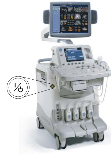
Figure 3. Power Switch Location
